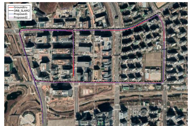
FIGURE 13 Trajectory estimates overlaid on the satellite map, which are performed on a portion of Urban 28 sequence (4.1 km) without restarts. The “Proposed 1” is the proposed visual localization using in-run PLM, and “Proposed 2” is the proposed visual localization using out-run PLM with a time gap of about 6 months; That is, the two LiDAR maps are built about 6 months apart. PLM, prior LiDAR map [Color figure can be viewed at wileyonlinelibrary.com]
