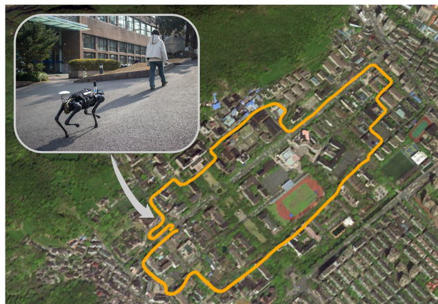
FIGURE 1 | Our proposed controller completes an automatic human-following tour in Zhejiang University assisted by a planner (Zhang et al. 2021) specifying its velocity. The robot finished the 3.1-km-tour within 37 min without human intervention, during which it encountered terrains such as slopes, vegetation, and gravel. Our controller demonstrates omnidirectionally accurate velocity tracking and long-term robustness.
