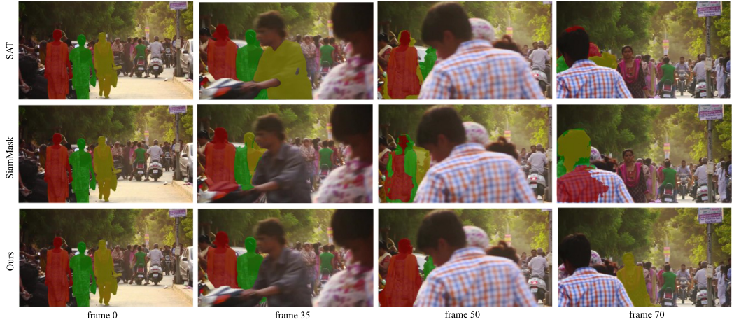
Fig. 6. Qualitative comparisons on DAVIS2017. Compared to SAT [3] and SiamMask [55], TMN is more robust to the target appearance changing and handles object occlusion better.
