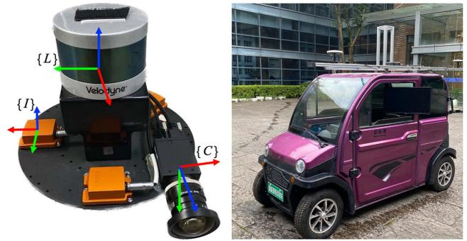
Fig. 6. Sensor rig and ground vehicle to collect YQ dataset.
