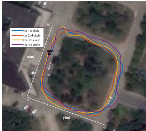
Fig. 7. Experiment 1: trajectory obtained by our VIO in the circle experiment. As there are uphill and downhill in circles, the trajectories of every circles are arbitrary due to the rough terrain.
