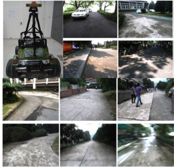
Fig. 6. Our toy vehicle VIO platform and the sample images captured by our platform (including different scenes, variation of illumination, moving objects, and blur).
