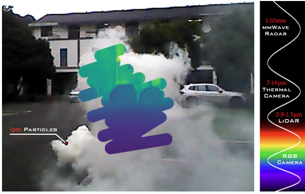
Fig. 1. Left: Our approach can provide high-quality depth estimation beyond the visible spectrum, unaffected by micrometer-sized particles. Right: Millimeter-wave radar and infrared thermal cameras have longer operational wavelengths than LiDAR and RGB cameras to penetrate atmospheric particles.
