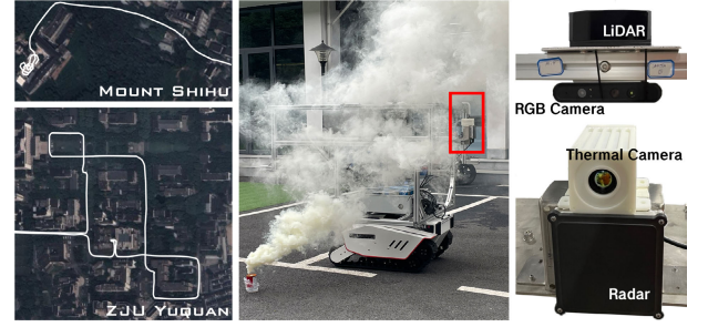
Fig. 6. ZJU-Multispectrum dataset. From left to right: data collection paths of ZJU-Multispectrum in Mount Shihu and Zhejiang University's Yuquan Campus, our vehicle equipped with multi-modal sensors, and the sensors mounted on the vehicle.
