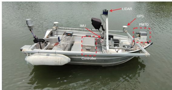
Fig. 1. An overview of the unmanned surface vehicle
