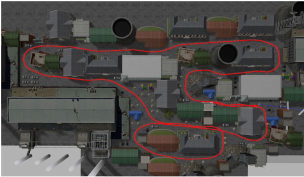
Fig. 5. The bird's-eye view of the synthetic Gazebo dataset. The 836 meter long groundtruth trajectory of the robot is shown in red. The maximum velocity of the robot was set to be 2.5 m/s.
