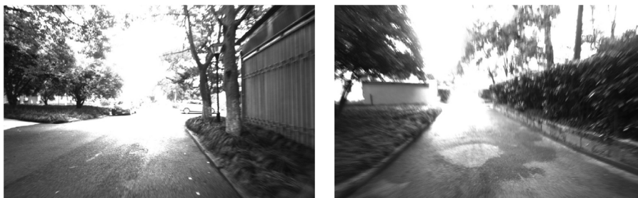
Fig. 14. Direct method fails due to light interference.
