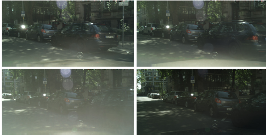
Fig. 5. Some images in Cityscapes Dataset [22] have severe brightness change due to the illumination and camera auto exposure and gain control.
