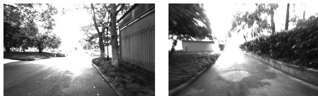
Fig. 6. Direct method fails due to light interference
