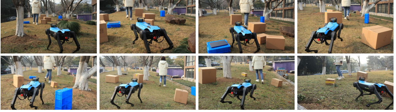
Fig. 12. Image flows of experimental trials on a lawn with undulating terrain and messy obstacles. From top to bottom: through multiple narrow passages with the closest distance gap 0.58 m and the maximum terrain slope 16.
