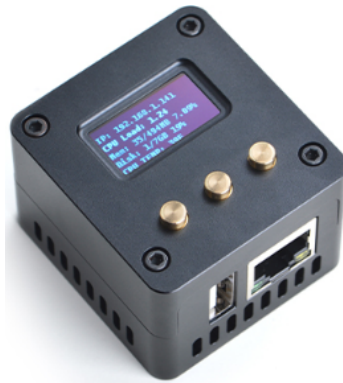
Fig. 2. AI-STBOX, an audio data acquisition and transmission equipment.
