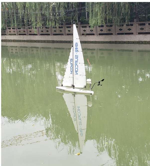
Fig. 9 The tested unmanned sailboat in pool
