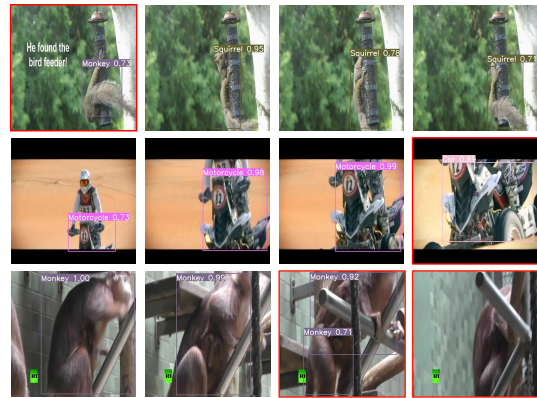
Fig. 6. Some failure cases caused by rare pose and occlusion. We mark the failure frames with red contour.
