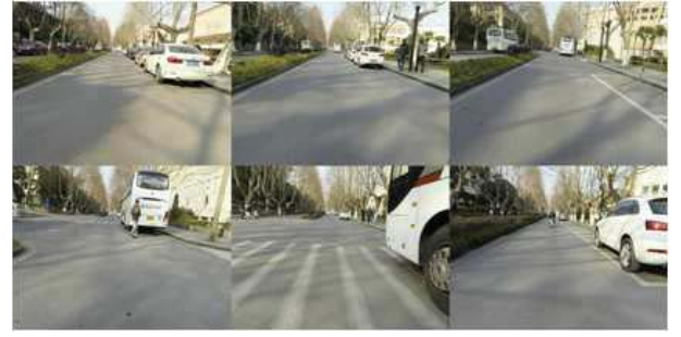
Fig. 7. Shadow road dataset containing shadows in the traversable regions. This dataset is a sequence containing 135 image frames, where all frames are labeled manually. It is captured by a monocular GoPro camera mounted on the robot with a frame rate of 5HZ. And the scene is a road lined with trees in our campus. There are many shadows of trees in sunny days.
