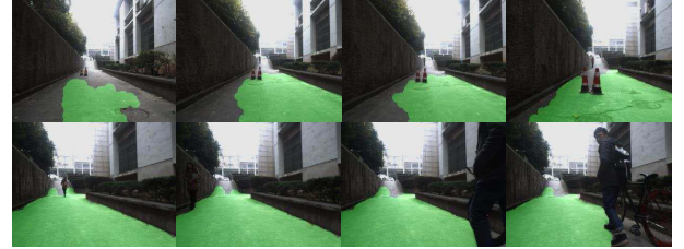
Fig. 22. Evaluation of the feasibility in robot navigation application when robot approaches an obstacle (top row), or moving obstacles approach the robot (bottom row).
