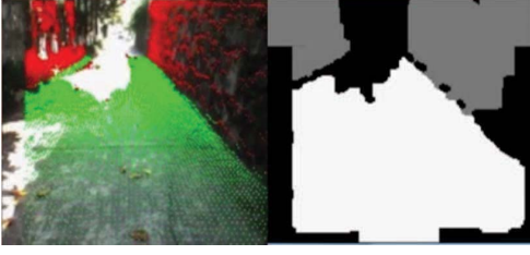
Fig. 5. The traversable region obtained by stereo vision system (left) and its corresponding mask (right).
