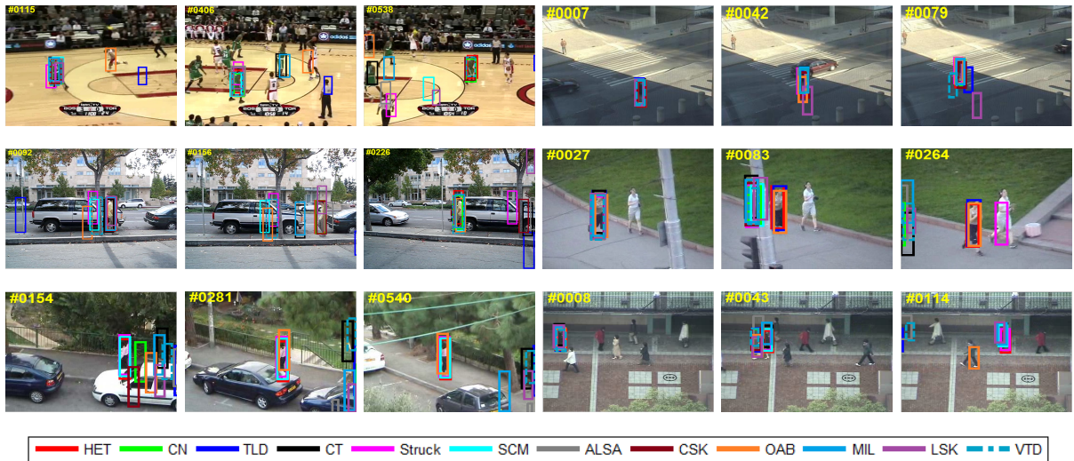
Fig. 8: Tracking results of 12 trackers (denoted in different colors and lines) on 6 image sequences. Frame indexes are shown in the top left of each figure in yellow color. Results are best viewed on high-resolution displays.
