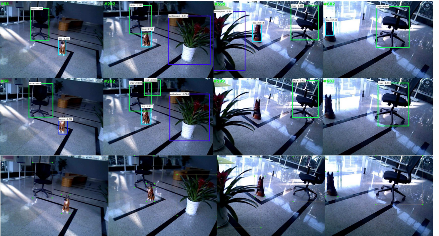
Fig. 6. Detection bounding boxes results in both methods. The first row is our method, the second row is Faster RCNN and the third row is Ground Truth.
