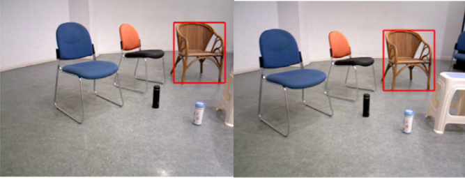
Fig. 3. Prediction from k th frame to p th frame. Left: Bounding box of the target chair in the k th frame. Right: The predicted bounding box of the target chair in the p th frame.
