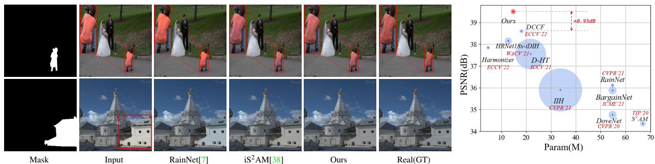
Figure 2. Left: Two challenging samples in image harmonization. Mask in column one and Red boxes represents the foreground. Right: Performance comparison with SOTA methods in terms of PSNR and model size. The circle size represents the floating-point number.
