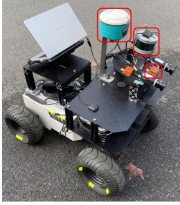
Fig. 5: The unmanned ground vehicle with self-assembled sensors rigidly mounted. Sensors with red box are used to collect YQ sequences in campus.
