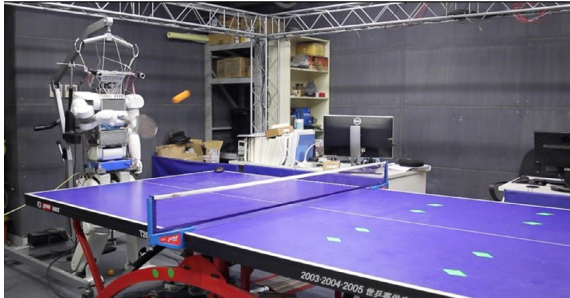
Fig. 1. Our Humanoid Ping-Pong Robot equipped with two onboard cameras with a baseline of 34 cm on the robot's head. It can walk by two legs and rally to human only with its onboard stereo vision system.
