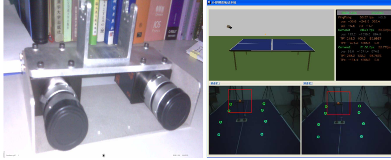
Figure 8. Hardware(left) and software(right) of the multi-camera system used for real case experiments. In the right-hand figure, the upper-left view shows the 3D pose of the multi-camera system in the virtual environment, while the lower views show the images from the system and the upper-right view shows the detailed 6DOF poses.
