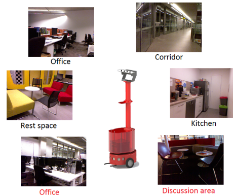
Fig. 1. Scene classification demonstration. The examples are captured in our university using the mobile robot. Our SS-CNN trained on SUN RGB-D dataset gives the predict labels below each image, without retraining for the completely new environment. Labels in black means correct classification. Two misclassified image are given with labels in red, while the predicted labels are in accord with human recognition to some extent.
