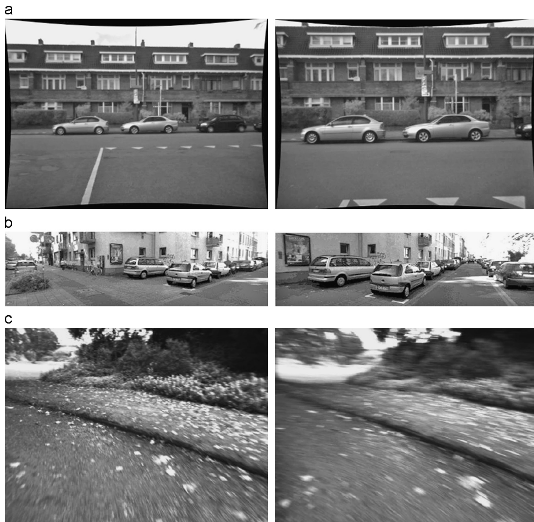
Fig. 9. Large image deformations due to the motion of vehicle.
