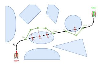
Fig. 3. An illustration of the path search process. The black path obtained by Dubins curve has several collision points  $p_c$ , which will be moved outside the collision with a safe distance, resulting the green path.
