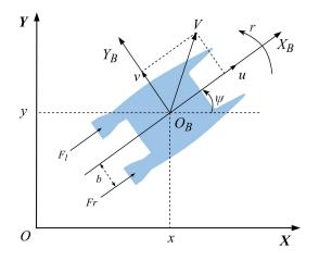
Fig. 2. USV earth-fixed and body-fixed coordinate frames.
