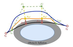
Fig. 4. An illustration of trajectory optimization. The orange path is sampled by  $A^*$  algorithm from original trajectory point  $v_{in}$  to  $v_{out}$ , and then the anchor points  $p_a$  are sampled. Finally, the blue path is generated by moving  $p_a$  to the safety guidance points  $\rho \in \mathcal{P}_t$ .
