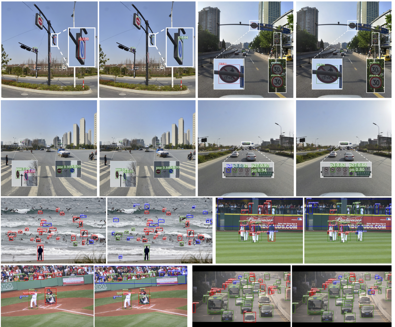
Fig. 8. Qualitative examples comparison between base model FPN and our EFPN on Tsinghua-Tencent 100K (row1&row2) and MS COCO (row3&row4). The left in each pair denotes FPN results, while the right denotes EFPN results. The red boxes represent false negatives, the blue boxes represent false positives, and the green boxes represent true positives. Detectors of traffic-signs and general objects both profit from EFPN on challenging small object detection.
