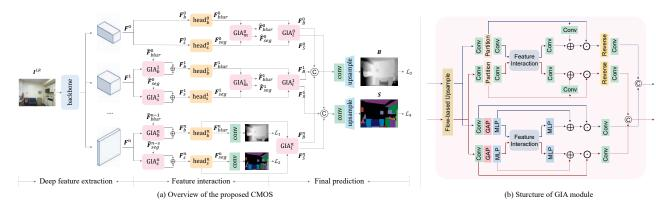
Figure 4. Architecture of CMOS and GIA. (a) Given an LR image, CMOS outputs the estimated blur map B and semantic map S simultaneously in the HR space. (b) GIA has two parallel streams to effectively interact features in both spatial and channel dimensions. It includes a flow-based upsample module to support inputs with different resolutions. If the input resolutions are the same, a feature alignment will also be performed through the learned flow field.
