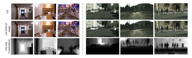
Figure 3. Original RGB images, the generated out-of-focus images and blur maps. The changes from dark to light in blur maps indicate that the corresponding out-of-focus image changes from clear to blur. The first three columns are images from NYUv2-BSR, and the last three columns are images from Cityscapes-BSR.
